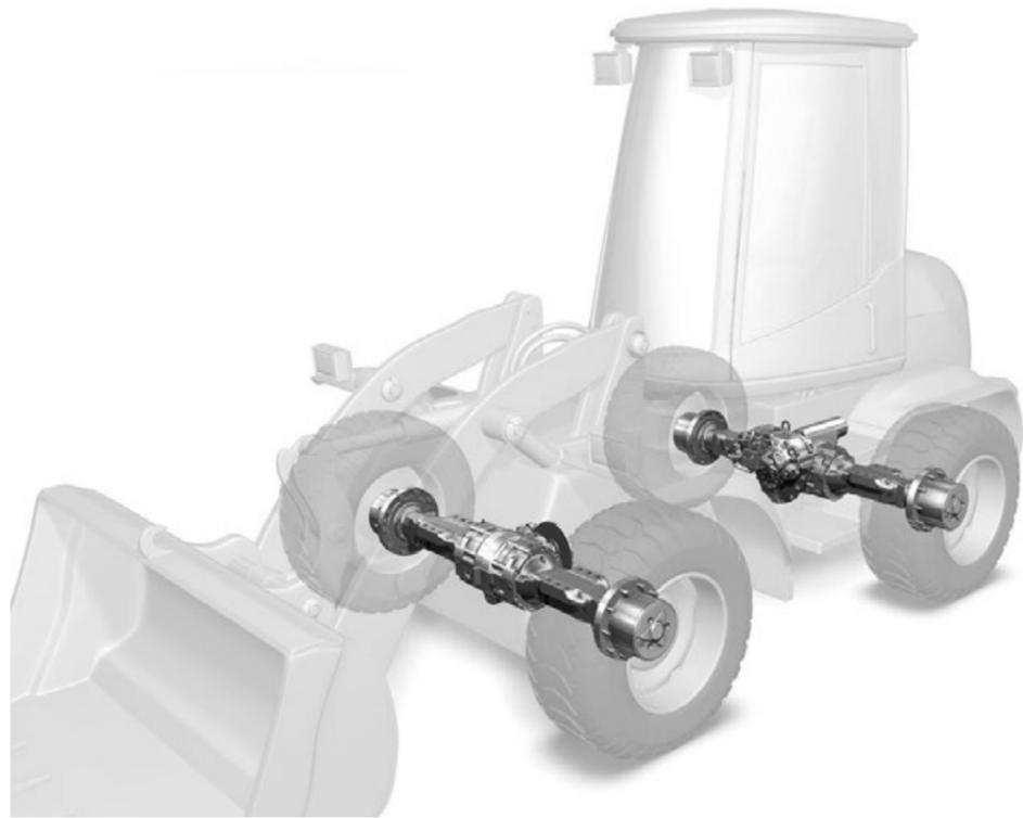
For the smaller range of articulated wheel loaders up to 10 tons empty vehicle weight ZF can offer the axle range MT-L 3055 in connection with the transmission AVG 185 or the new CVT transmission 2 HC 85 for the adaption of the hydrostatic engine. These axles in connection with a possible mounted service and parking brake (BHF) have a very compact design.
